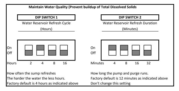
Water quality is maintained by periodically draining and filling the reservoirs. The harder the water the shorter the cycle time. The softer your local water is the longer (hours) the refresh cycle can be. If you see white powder developing on the paper media, shorten the refresh cycle.
