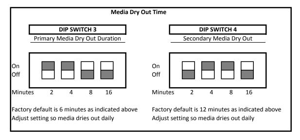
Paper media should dry out completely at least one time each day. When indoor thermostat setting is reached, the water pump(s) turn off but the fan(s) run for a set period of time based on the dip switch settings. This allows the paper media to dry out. This prevents bacteria or algae growth on the pads. The drier the climate, the less time is needed to run fans to dry out. The more humid the climate the longer the fans need to run to dry out media.
