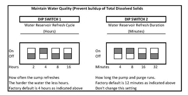
Water quality is maintained by periodically draining and filling the reservoirs. The harder the water the shorter the cycle time. The softer your local water is the longer (hours) the refresh cycle can be. If you see white powder developing on the paper media, shorten the refresh cycle.
